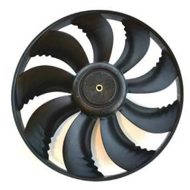
The 30XB and 30XBP utilize Carrier's 6<sup>th</sup> generation Flying Bird<sup>™</sup> fan technology, engineered for maximum efficiency, super low noise, and wide operating range. The fan includes Carrier patented rotating shroud technology and back-swept blades with a unique wave-serration trailing edge inspired from nature.
